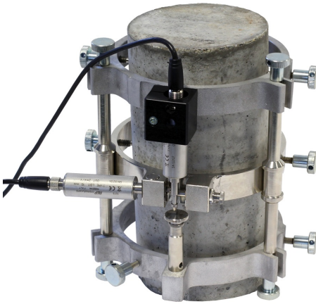
Compressometer/extensometer model 55-C0221/E fitted with two high precision displacement transducers LDT type, 0,001mm x 10mm
